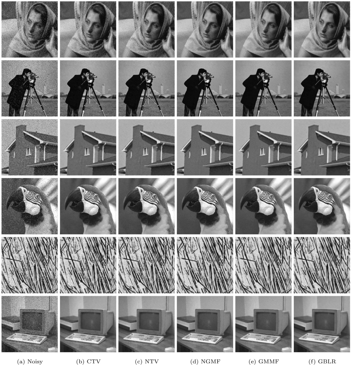
Fig. 5. Restored images by different methods with \gamma = 5 . (a) noisy image, the results of (b) CTV, (c) NTV, (d) NGMF, (e) GMMF, and (f) GBLR.
