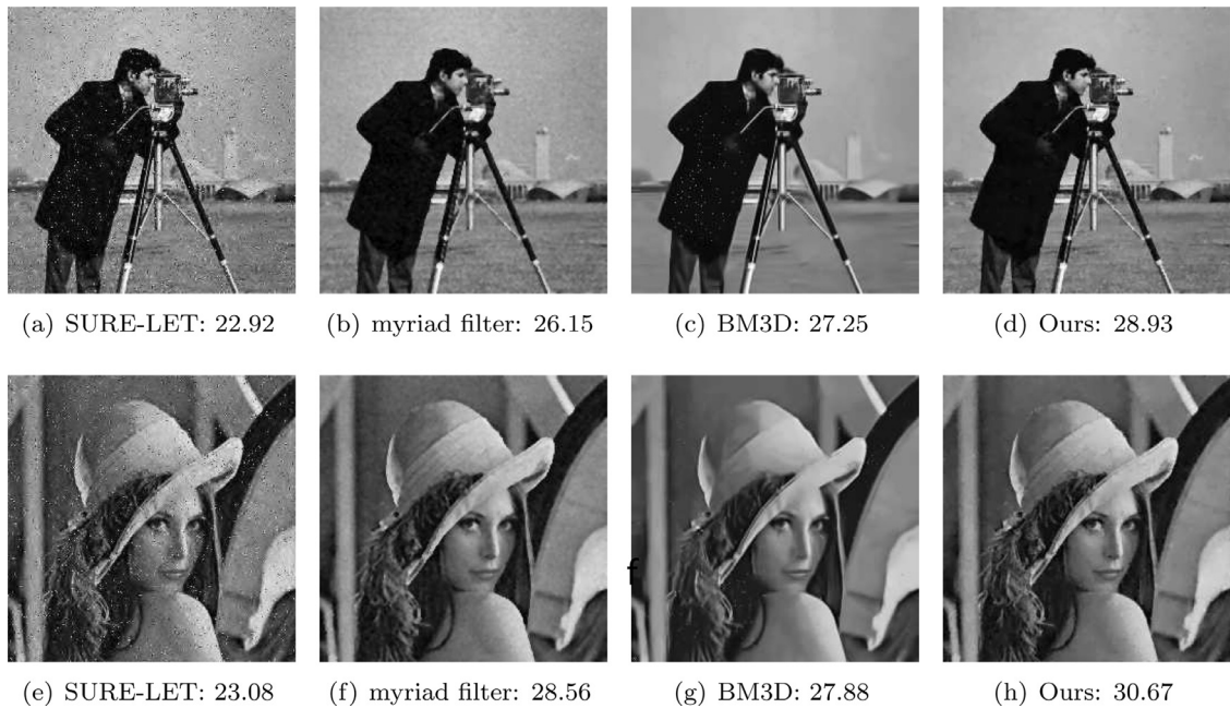
Fig. 9. Recovered images of different methods for removing Cauchy noise with the noise level \xi = 0.02 . The number under images represents the PSNR (dB) of images. First column: restored images by SURE-LET; second column: restored images by the myriad filter; third column: restored images by BM3D; fourth column: restored images by our method.
